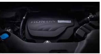
3.5-liter direct injected i-VTEC® 24-valve SOHC V6 engine
