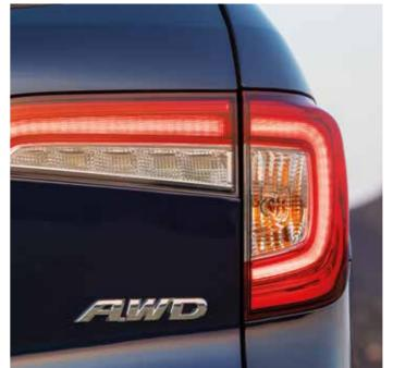
The rear receives new taillights with amber turn signals and LED reversing lights.
