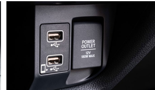
12 V power outlet and 2 USBs for smartphones connectivity or simply charging your devices.
