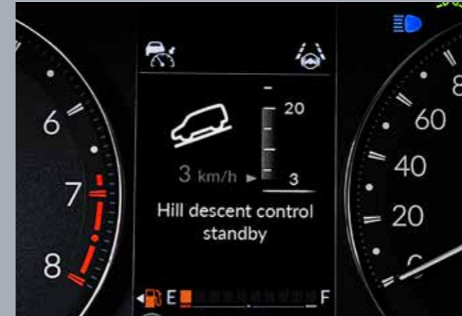
Hill Descent Control (HDC), automatically controls the speed between 0-20 km/h when descending hills
