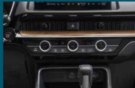
A striking metal honeycomb mesh accent stretches across the dash. A design element that debuted on the 2022 Civic, the honeycomb trim serves both form and function, creating a dramatic visual dividing line between the audio, information displays and climate controls, while the flow-through design conceals the air vents that might otherwise mar the uncluttered and harmonious look of the dash.
