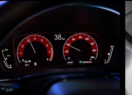
**Full-color LCD panel:** The All-New Civic features first all-digital LCD instrument display. Measuring 10.2 inches, the high-definition full-color LCD panel displays a variety of information, all customizable from the steering wheel.
