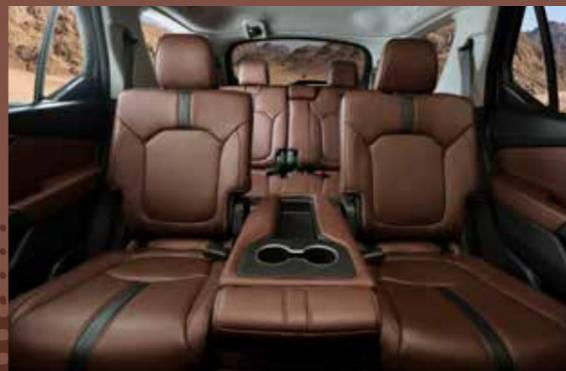
In the second row, the middle seat can either be folded down, to provide an armrest and two cup holders for convenience. The seat can be completely removed, allowing a walk-through access to the third-row
